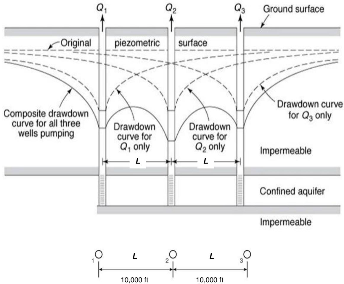
**ASR Conceptual Wellfield Model using Theis Superposition Method**
